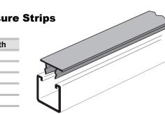
Elevator Guide Rail Insert Closure Strips, or snap-in covers, keep construction debris out. Exceptionally useful during inserts installation in masonry wall. Dark grey color, PVC, 1-3/8" wide, 1/16" thick.
